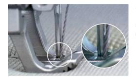
Sewing of very dense or very hard materials leads to crushing of the thread between the sewing fabric and the scarf edge during the needle down stroke.
