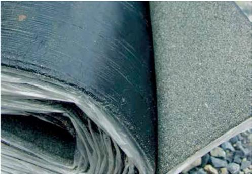
Bitumen-coated roofing felt
