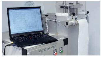
Measurement of penetration force and mechanical work
